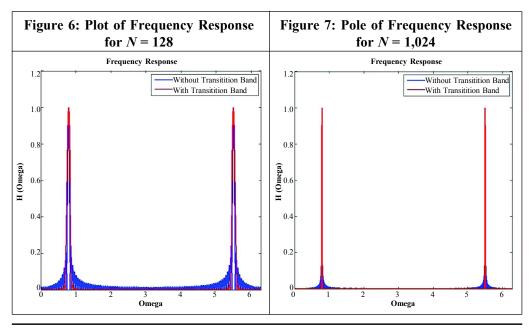
N = 128 and 1,024. Table 2 shows the spectral contents in the passband and the stopband of the filter response (Jim, 2007; and Pushpavathi, 2020).
