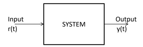
The output not only depends on the input applied to the system for  $t > t_0$ , but also on the initial conditions at time  $t = t_0$
