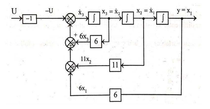
Represent the differential equation given below in a state model
