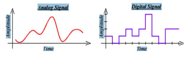
Infinite versus finite number of states → Analog = Digital + Every point in between.
